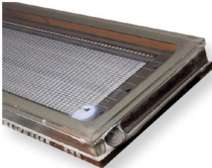
Note that the discolored area on the display that looks like a "burn mark" is actually normal and does not indicate a problem. The problem is the missing glass bulb at the lower right corner of the display.
