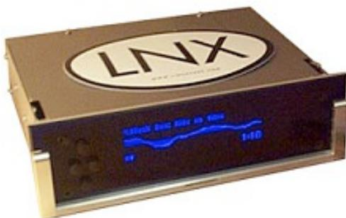
**The empeg Car Mark 1** was released in the late summer of 1999, and fewer than 400 units total were shipped to customers. The Mark 1 had space for two 2.5" laptop hard disks, and it had 8 megabytes of RAM for running software and caching songs. USB and Serial were the connections available to interface with your PC. It had a plain faceplate with four simple buttons. It had a built-in FM-only tuner. Despite being a "first product", its design was very advanced. The hard
