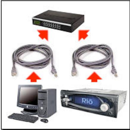
In this configuration, the PC (or multiple PCs) and the car player are connected to an ethernet hub or switch with standard "straight-through" 10baseT network cables. This, of course, requires that the PC has an ethernet adapter card installed and working.
